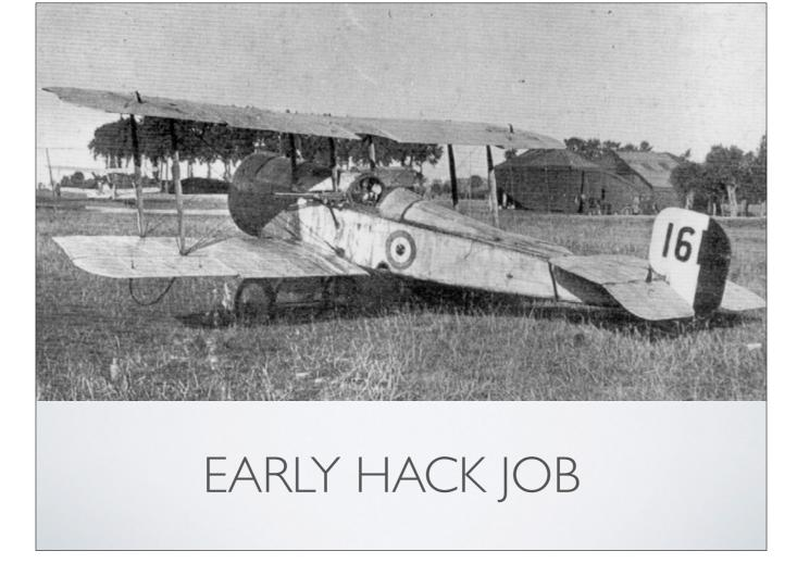
the difficulty with mounting a gun on a plane is to avoid the propellor arc (otherwise you crash and die). very first hack was to just mount the gun at an angle on the side. Bristol Scout C, flown by Lanoe Hawker, july 15 1915 shot down 3 German planes
